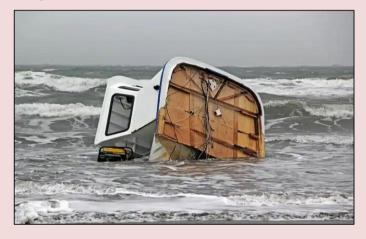
F/V EVENING: Oct 12, 2023--Off coast of Grays Harbor, WA: 43.4 ft, wood hul, built in 1941, tuna troller with 2 POB and a dog, was returning to port after 2 days of tuna fishing. The weather was very rough with a quartering sea. Vessel listed sharply and capsized. Deckhand made it to the liferaft but skipper and the dog were never seen again. Deckhand survived 13 days in the liferaft until being picked up by a Canadian Fishing Vessel 70 nm NW of Cape Flattery, WA.
